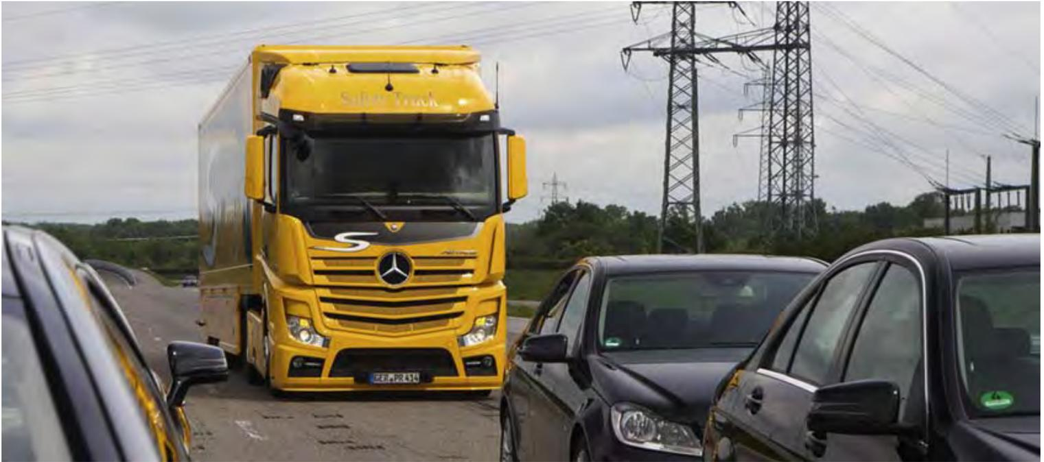
The new "Active Brake Assist 3" now independently applies the full brakes if a stationary object is detected ahead.
